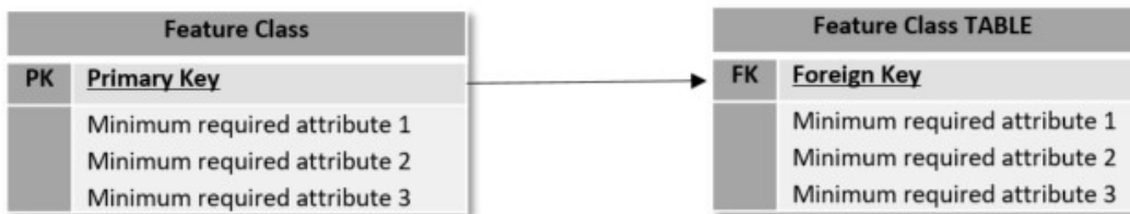
Figure 3b. Feature class with associated external business table, linked by a common Primary Key (PK) and Foreign Key (FK).
